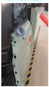
Insert water into the inlet of the filling tube on the rear side of the cover.
